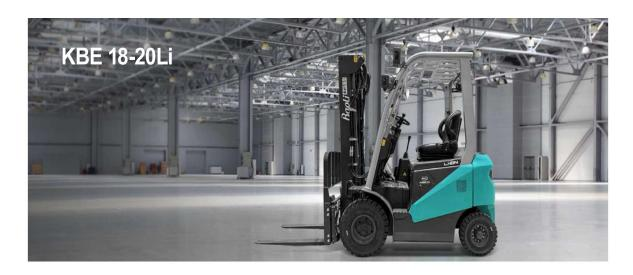
The KBE 18Li and KBE 20Li, with a load capacity of 1.8 to 2.0 tons and a maximum lifting height of 6.5 meters, are ideal for logistics and industries, especially in indoor spaces, thanks to their zero emissions and low noise levels. These trucks excel in light to medium-duty operations, featuring a compact design for easy handling in narrow spaces.
