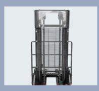
Mast can offer better rigidity and stabilit in comparison with C-shaped steel channels
