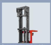
i ne mast chain with a safety factor of 10 time is equipped with a chain safety switch
