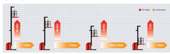
A series order picker is available with advanced intellispeed system, which smoothly coordinates travel speeds and load height. Compared to conventional speed control, intellispeed maximizes truck speed as the platform rises, capitalizing on an area of opportunity for providing faster travel between picks.
