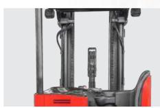
The optimized design of the wide-view mast enables the operator to get a better view, and improves the operation safety.
