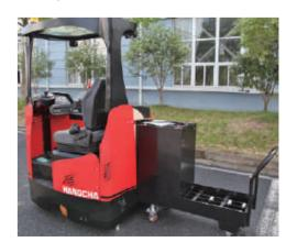
Standard configuration: Battery side roll-out + trolley(optional)
