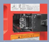
Charging plug inside operator's compartment, this eliminates the need to disconnect the plug from battery, enhancing ease of operation (Std.)
