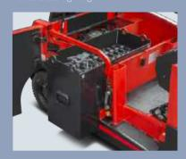
Battery side roll out is taken as the standard configuration in order to easily and fast replace the battery
