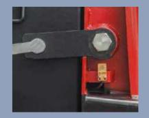
The locking device of the battery is provided with the safety protection function. Only if the locking device otated in place, the tractor can tra-
