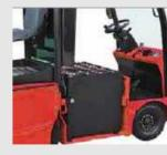
Side change battery design is convenient for changing battery
