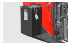
The lateral removal of the battery provides easier maintenance and is applicable to continuous operating conditions.
