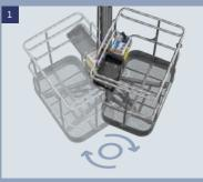
Basket: can be rotated left and right at an Angle of 140°
