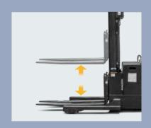
Standard configuration of lifting and lowering stepless speed regulation realizes more accurate operation of the fork
