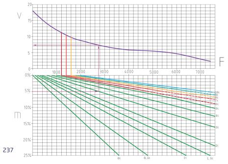
v=speed (km/h), m=incline (%), F=drawbar pull (N)
