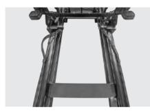
A new optimized lifting system enables the operator's wider view through the mast and excellent line of sight.
