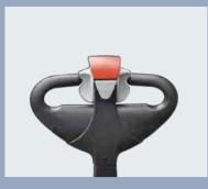
The unique lighted creep speed driving function allows the truck to move at slow speed more conveniently.
