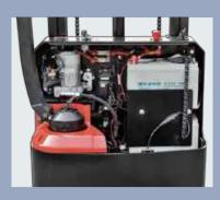
Fully opened hood, easy accessibility of a components, is easy for service
