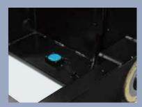
The tilt sensor prevents the vehicle from tipping due to excessive slope and ensures operator safety
