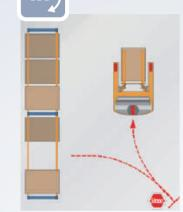
In the mode of 180-degree steering, the truck must be reversed until it stops completely, and the direction must be switched before the truck can travel forward, with lower efficiency.
