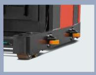
Rail guidance rollers (Opt.) can be fitted to th truck for VNA working
